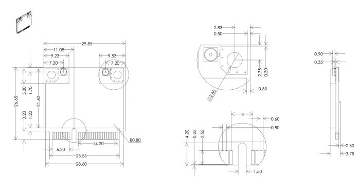
\* Measures in millimeters (mm). Tolerance below 0.15mm unless otherwise specified.
