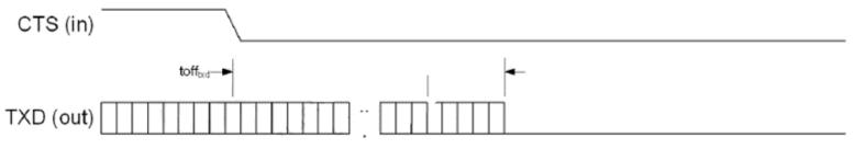
Figure 8-1: HCI UART transmit flow control timing
