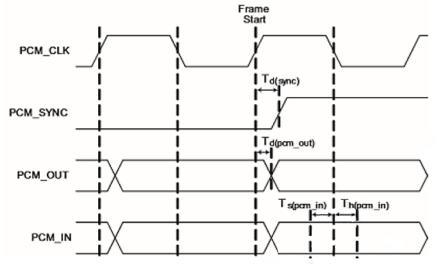
Figure 8-3:PCM interface timing diagram (slave)
