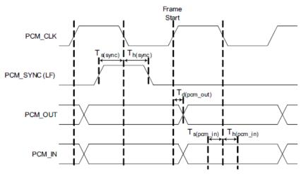
Figure 8-4: PCM interface timing diagram (master)
